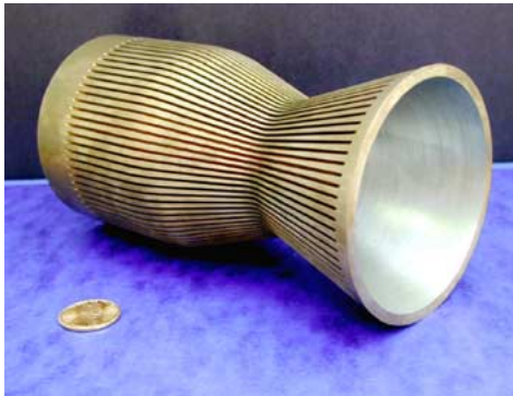
Figure 26 NASA's main combustion chamber made of copper based alloys with cooling channels.
