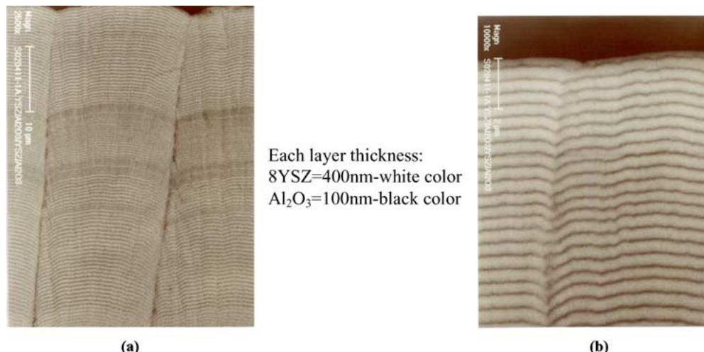
Figure 24 SEM photographs showing nanolayered 8YSZ (white color) and Al 2 O 3 (black color) coatings produced by co-evaporation of two ingots: 8YSZ and Al 2 O 3 in the EB-PVD chamber.
